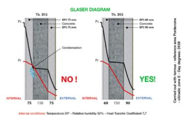
Glaser diagram created on walls of equal thickness with different distribution of the insulation.
